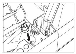
Attach the Feed Roller. Align the notch on the roller axis with the hole on the roller.
