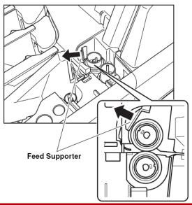
Pinch the Separation Roller at the rim and the fixing lever, and then remove it with pressing the Separation OFF Mode Button.
