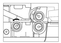
**5** Pinch the Feed Roller at the rim and the fixing lever, and then remove it.
